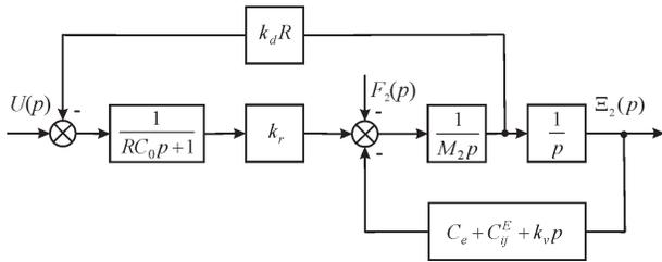
Figure 3: Structural diagram of piezo actuator at elastic-inertial load.
