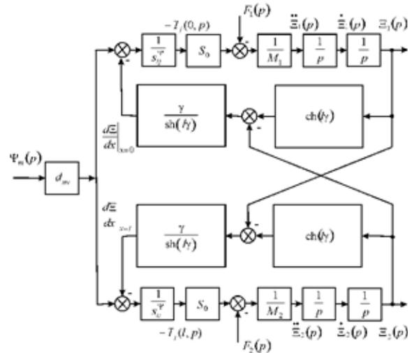
Figure 1: Structural diagram of actuator for nanobiotechnology.
