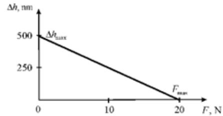
Figure 4: Mechanical characteristic of transverse piezo actuator.
